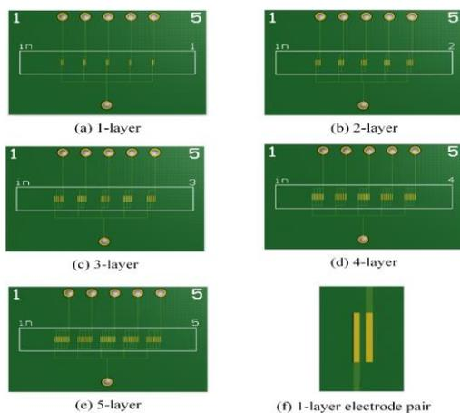
**Figure 1:** The five types of electrode and the magnified version of the 1-layer electrode. The gold-colored patterns are  $100\mu\text{m} \times 1\text{mm}$  and they are separated  $100\mu\text{m}$  away.
