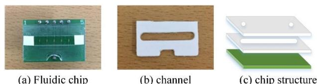
**Figure 2:** Electrode Fluidic chip. The channel width and length is  $4 \times 23\text{mm}$  (b). The chip is constructed with  $100\mu\text{m}$  polycarbonate,  $400\mu\text{m}$  double-sided tape, and PCB substrate from the top to the bottom (c).
