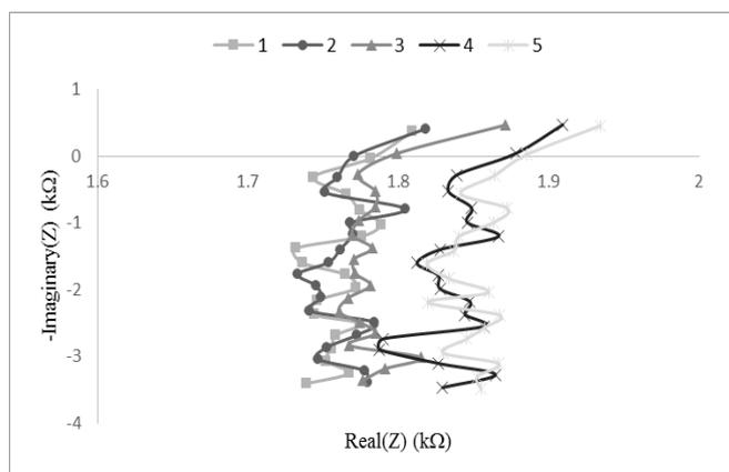
Figure 6: Impedance variation of 5-layer electrode pairs
