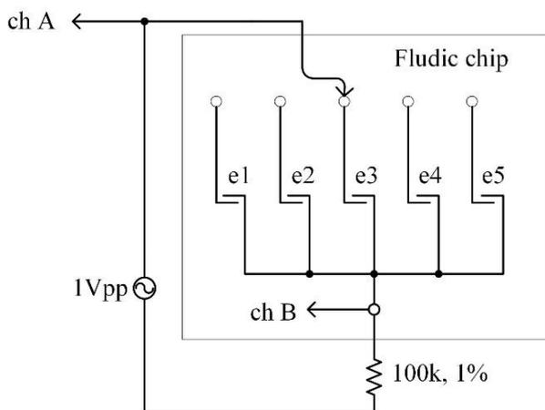
Figure 3: Impedance measurement circuit diagram.
