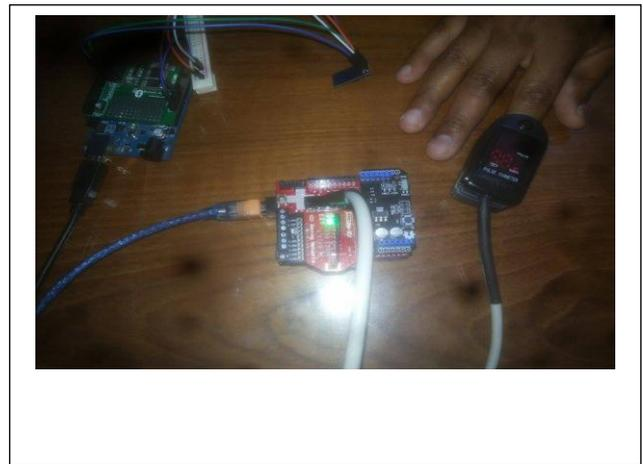
Figure 3: Pulses and Oxygen in Blood Sensor (SPO2).
