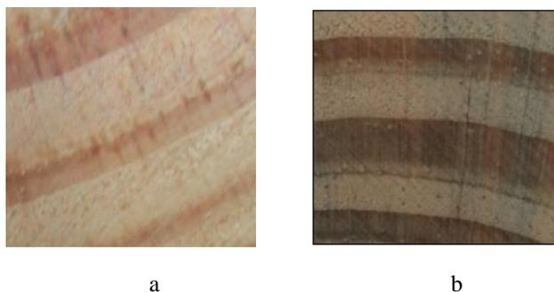
**Figure 1:** Contact surfaces of sound sample (a) and blue-stained sample (b)
