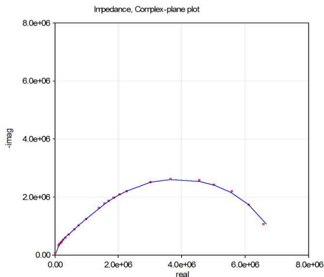
**Figure 4:** Imaginary component of the impedance ( $Z_i$ ) as a function of the real component ( $Z_r$ ) for blued MPW. Experimental (dashed) and theoretical (continuous lines) curves deduced from the double DCE model.
