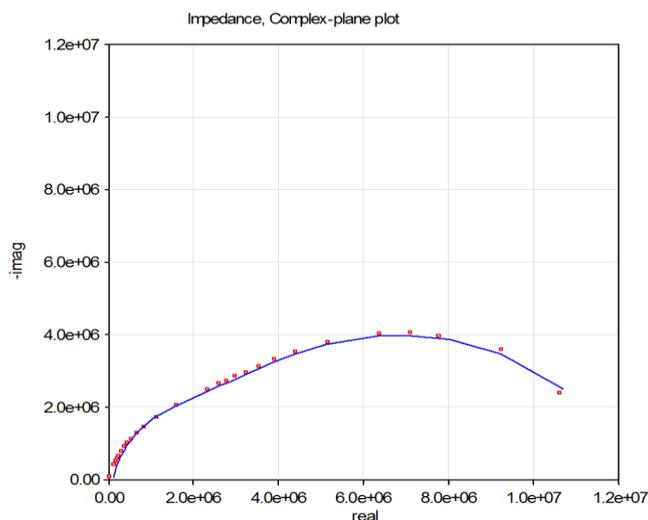
**Figure 5:** Imaginary component of the impedance ( $Z_i$ ) as a function of the real component ( $Z_r$ ) for blued MPW after drying. Experimental (dashed) and theoretical (continuous lines) curves deduced from the double DCE model.
