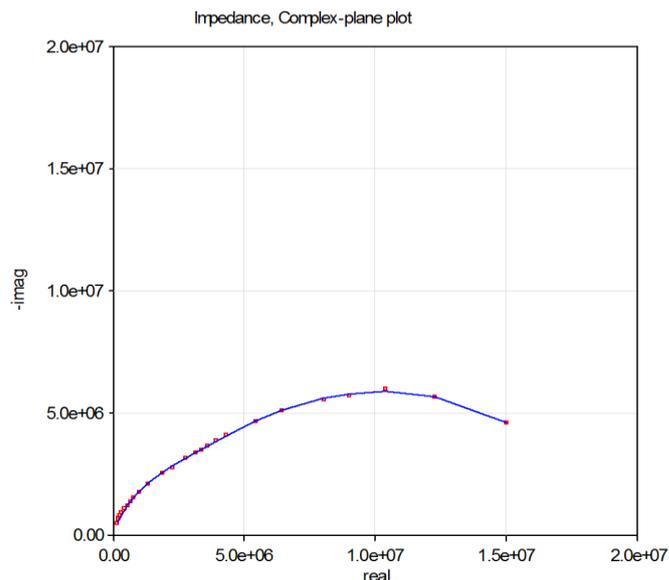
**Figure 3:** Imaginary component of the impedance ( $Z_i$ ) as a function of the real component ( $Z_r$ ) for sound MPW. Experimental (dashed) and theoretical (continuous lines) curves deduced from the double DCE model.
