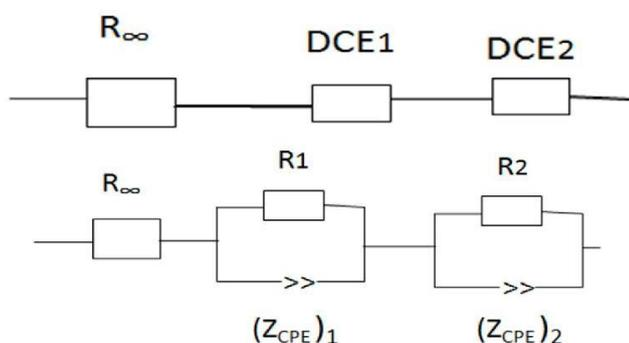
**Figure 2:** Equivalent circuit of the double-DCE model (ZARC)
