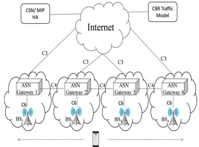
**Figure 3:** Experimental architecture
