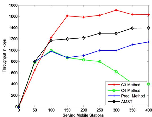
**Figure 8:** ASN Gateway's Average Throughput vs Serving MSs
