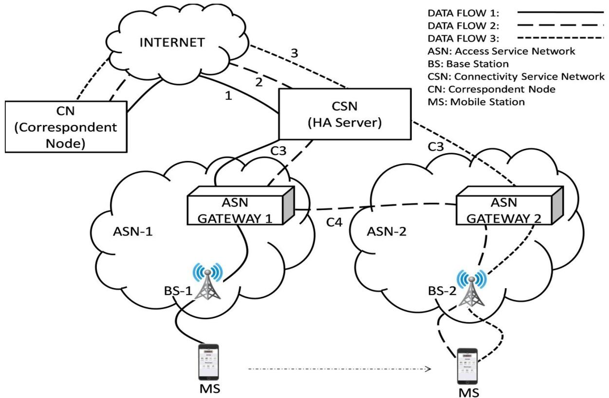
**Figure 1:** ASN connected and CSN connected Mobility in WiMax
