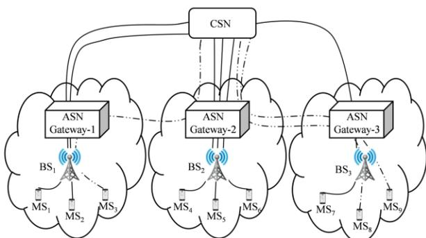
**Figure 2:** WiMax Network using three ASN Gateways
