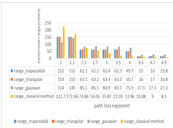
Figure 7: fuzzy logic based transmission range vs. path loss exponent
