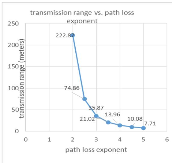
Figure 6: transmission range vs. path loss exponent
