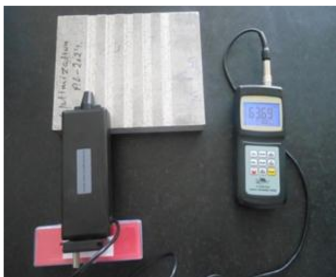
Figure 3: ITI surftest to measure surface roughness
