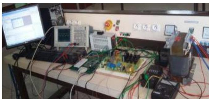
**Figure 18:** Hardware implementation full scheme of the uncontrolled three phase rectifier plus boost converter with its intermediate interface
