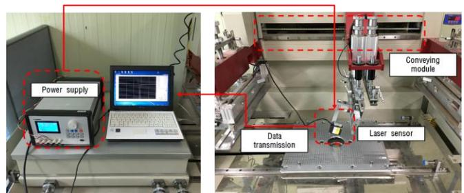
**Figure 8:** Deflection measurement system
