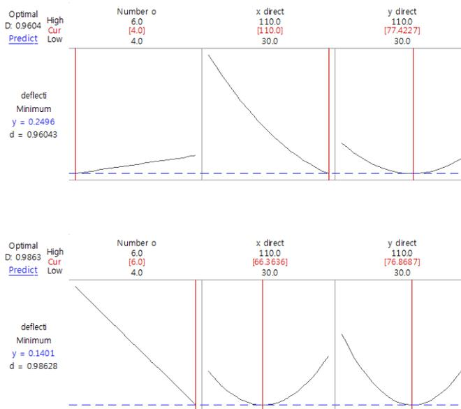
Figure 11: Optimum spacing obtained using a response optimizer
