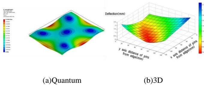
**Figure 4:** Results and deflection pattern obtained with five support pins
