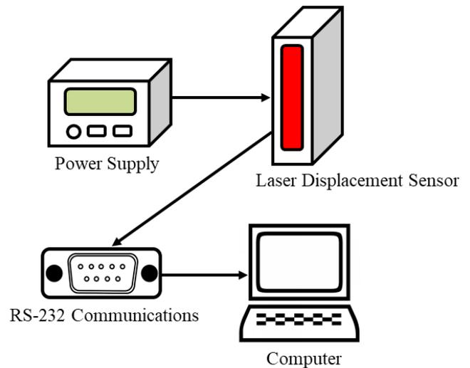
**Figure 7:** Experimental setup schematic diagram
