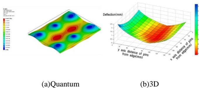
**Figure 5:** Results and deflection pattern obtained with six support pins
