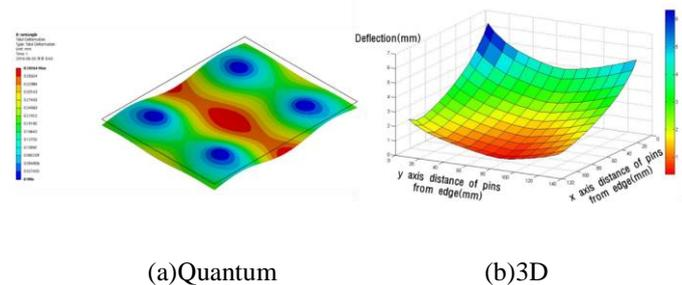
Figure 3: Results and deflection pattern obtained with four support pins
