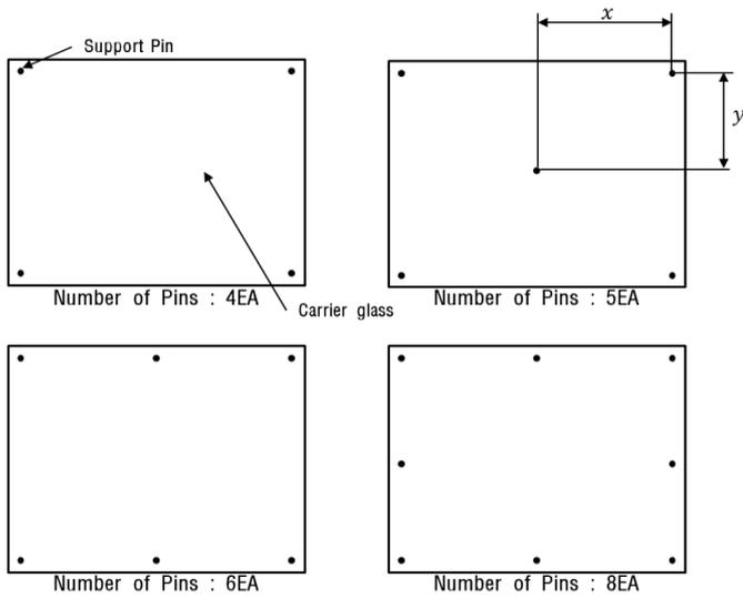
Figure 1: Pin arrangement for various numbers of pins
