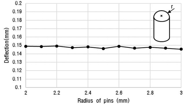
Figure 2: Glass deflection for different pin tip diameters
