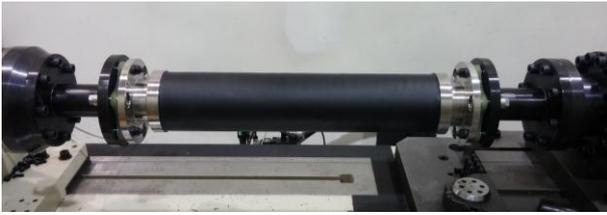
**Figure 14:** Long shaft coupling durability test result
