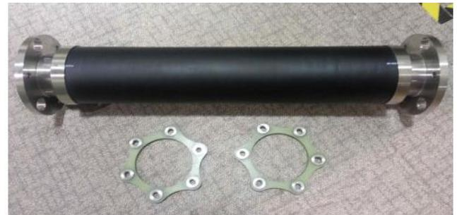
**Figure 13:** Prototype for the long shaft coupling durability test
