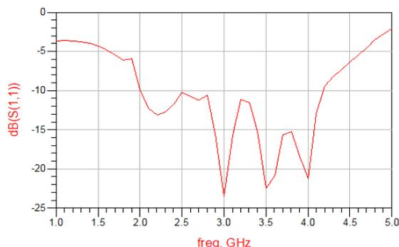
**Figure 6:** Input return loss  $S_{11}$
