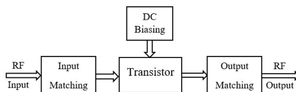
**Figure 1:** Components of RF Power Amplifier
