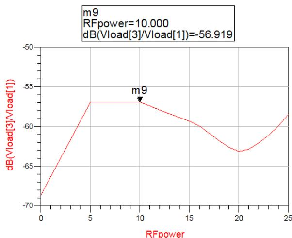
**Figure 7:** IMD3 vs RF power
