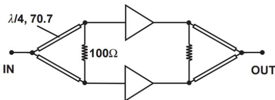
**Figure 2:** Two Stage Amplifier using Power Combining Technique [9]
