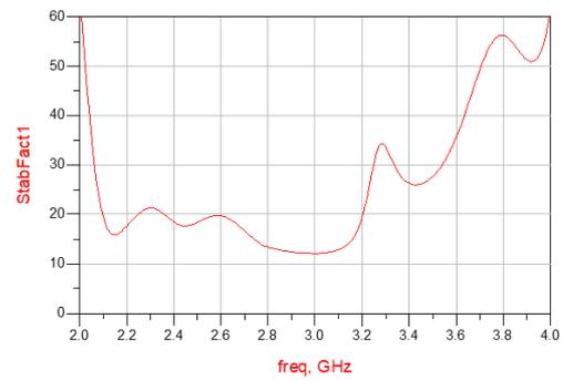
**Figure 4:** Stability of power amplifier
