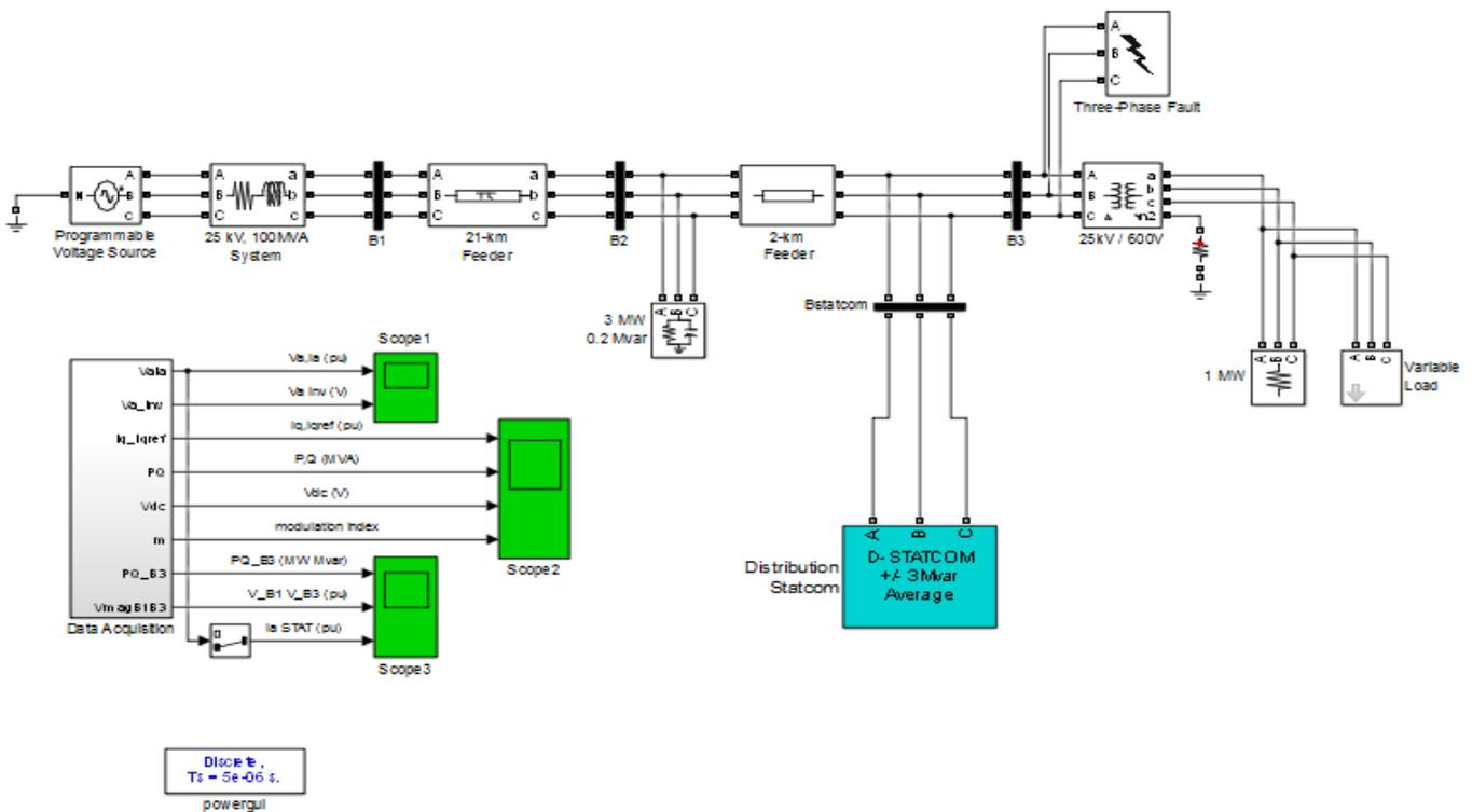
Figure 1: Distribution line with D-STATCOM and Three-phase fault.
