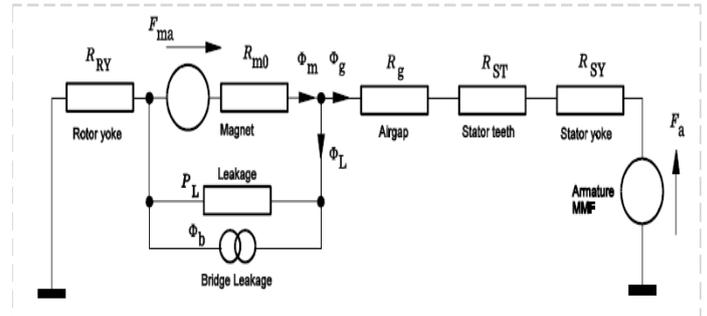
Figure 4: Non-linear equivalent circuit
