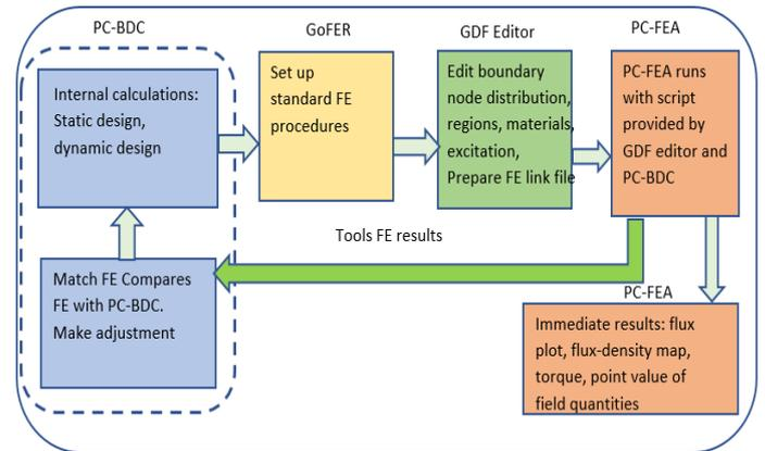
Figure 9: Finite element process with SPEED
