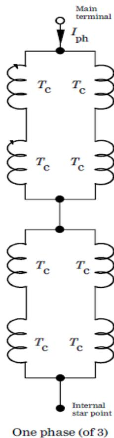
**Figure 13:** Stator equivalent circuit (one phase)
