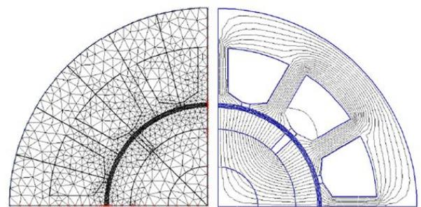
Figure 10: Finite-element mesh for PMBLDC motor and Magnetic field (open circuit)-SPEED
