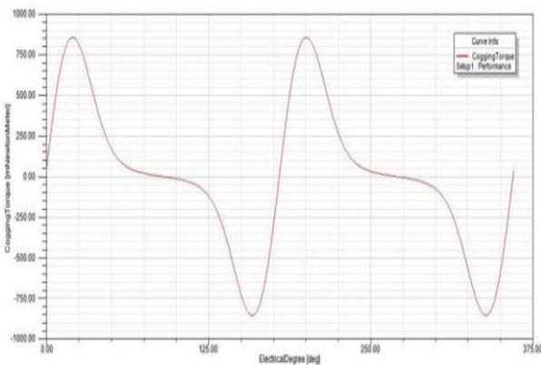
Figure 8: Cogging torque of PM Brushless motor
