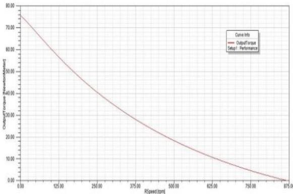
Figure 7: PM Brushless motor Torque
