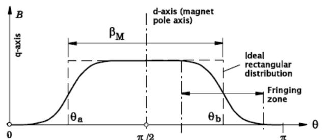
Figure 5: Airgap flux distribution
