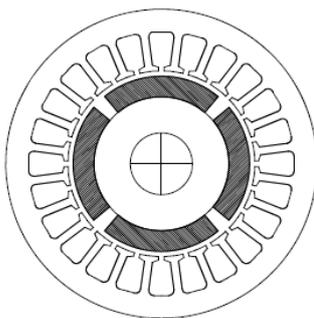
Figure 1: Brushless permanent-magnet motor
