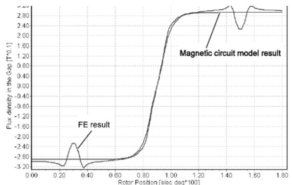
Figure 11: Comparison of finite-element and magnetic-circuit model
