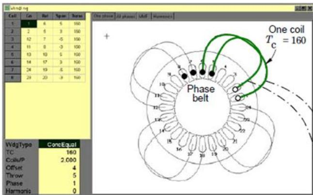
**Figure 12:** Motor stator winding schematic
