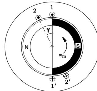
Figure 2: Back EMF generation in PMBLDC motor
