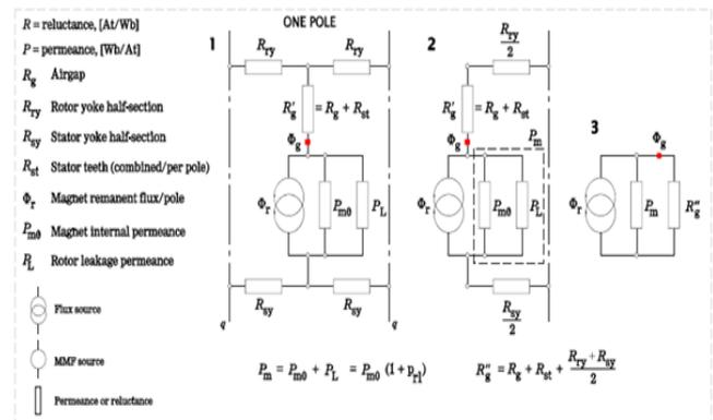
Figure 3: Magnetic equivalent circuit
