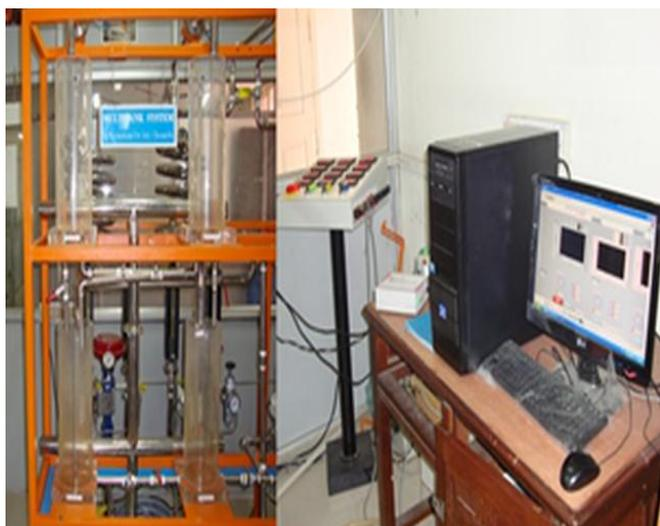
**Figure 2:** Experimental setup of the quadruple-tank process.
