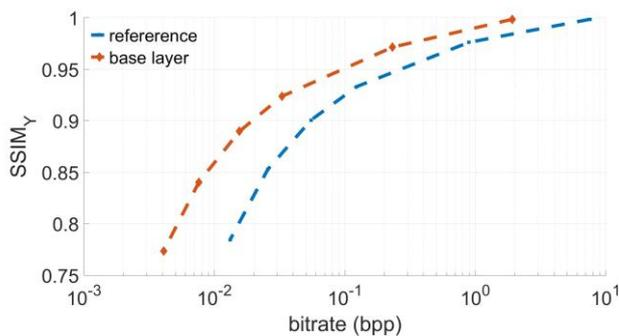
**Figure 10:** Rate-distortion curves showing  $SSIM_Y$ (dB) vs  $bitrate$  (bpp) for light field *Danger de Mort*.
