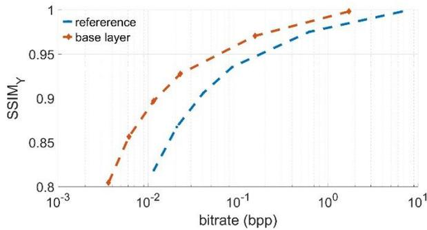
**Figure 8:** Rate-distortion curves showing  $SSIM_Y$ (dB) vs  $bitrate$  (bpp) for light field *Bikes*.
