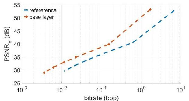
**Figure 7:** Rate-distortion curves showing  $PSNR_Y$  (dB) vs *bitrate* (bpp) for light field *Bikes*.
