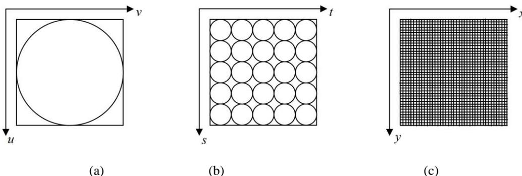
**Figure 1:** Conceptual model for a light field camera. (a) Main lens; (b) Rectangular microlens array; (c) Digital photosensor.
