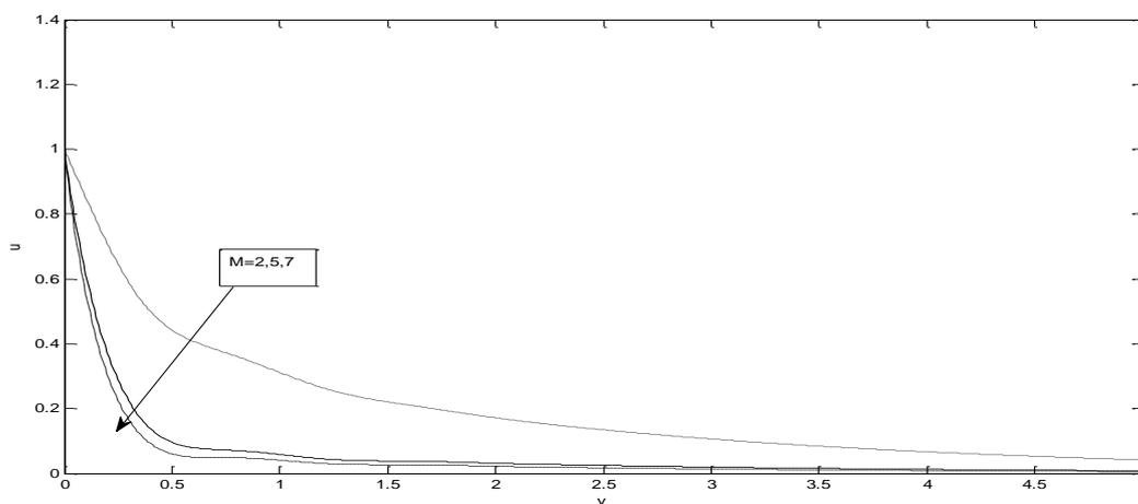
**Figure 2:** The velocity profile  $u$  against the displacement variable  $y$  for  $\alpha=.03, Pr=.71, Gr=5, Gm=2, Sc=.3, Kr=.5, Nr=.5, S=.05, n=.7, k=1.5, A=.3, \alpha=-.03, \epsilon=.02$
