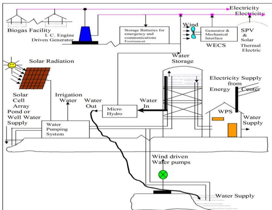
**Figure 3:** Schematic diagram of rural energy center to harness renewable energy sources in the Hybrid Form.
