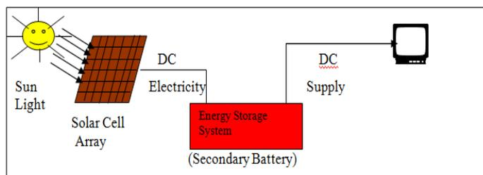
**Figure 2(a):** System Using Solar Cell Arrays and Energy Storage
