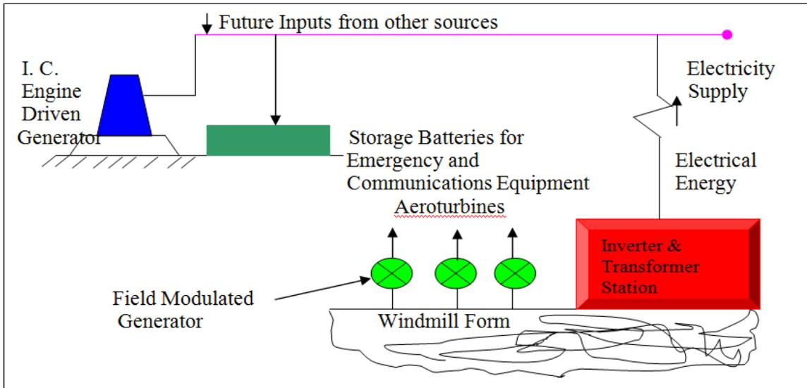
Figure 1: Schematic of the Electrical Station
