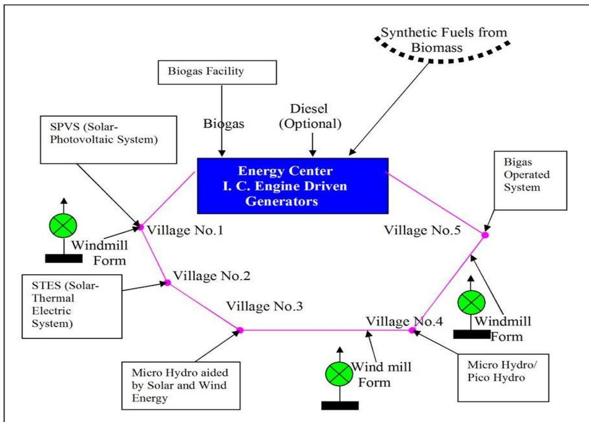
Figure 4: Scheme to energize a small cluster of Villages
