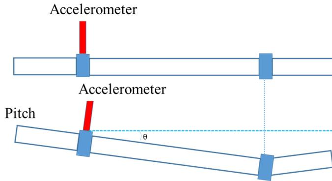
Figure 3. The Accelerometer on water supply pipeline
