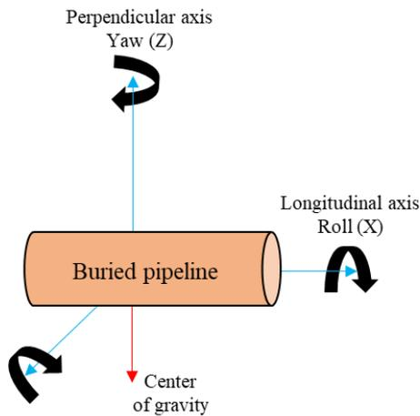
Figure 1. The Roll, Pitch and Yaw of buried pipeline
