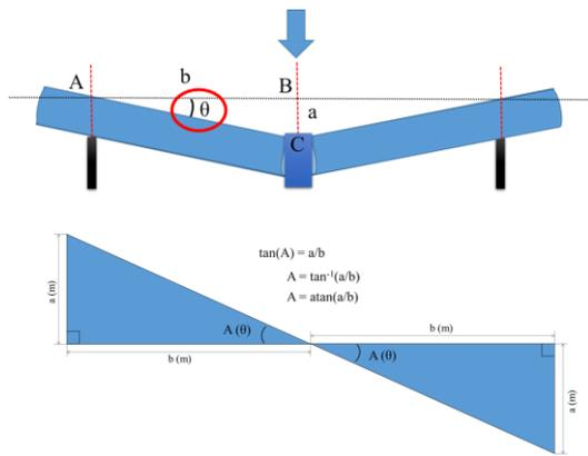
(b) Pipeline displacements calculation
