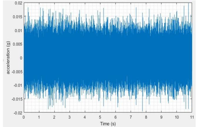
Figure 4. The magnitude of acceleration values in water pipeline during leakage
