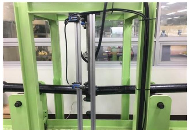
(a) Bending test equipment
