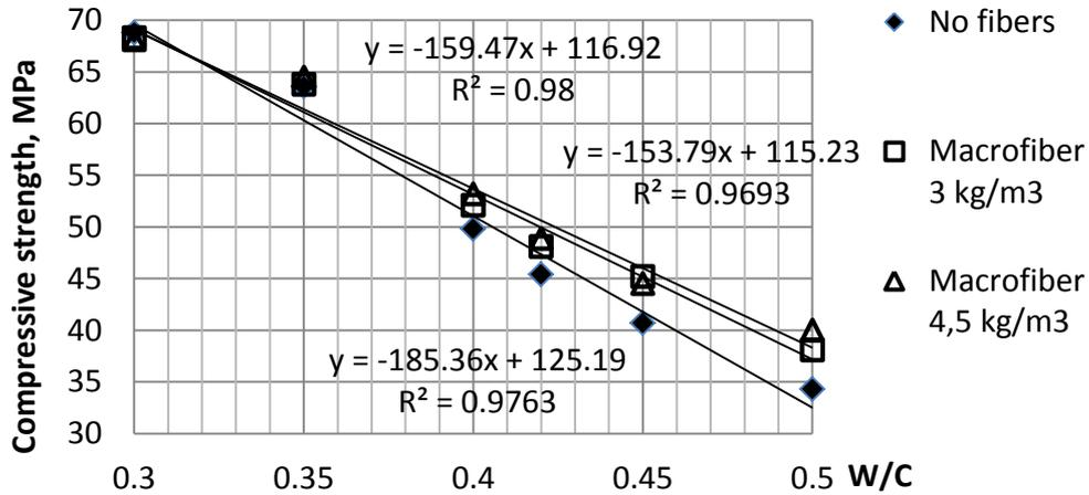
**Figure 3:** The concrete compressive strength at the age of 28 days
