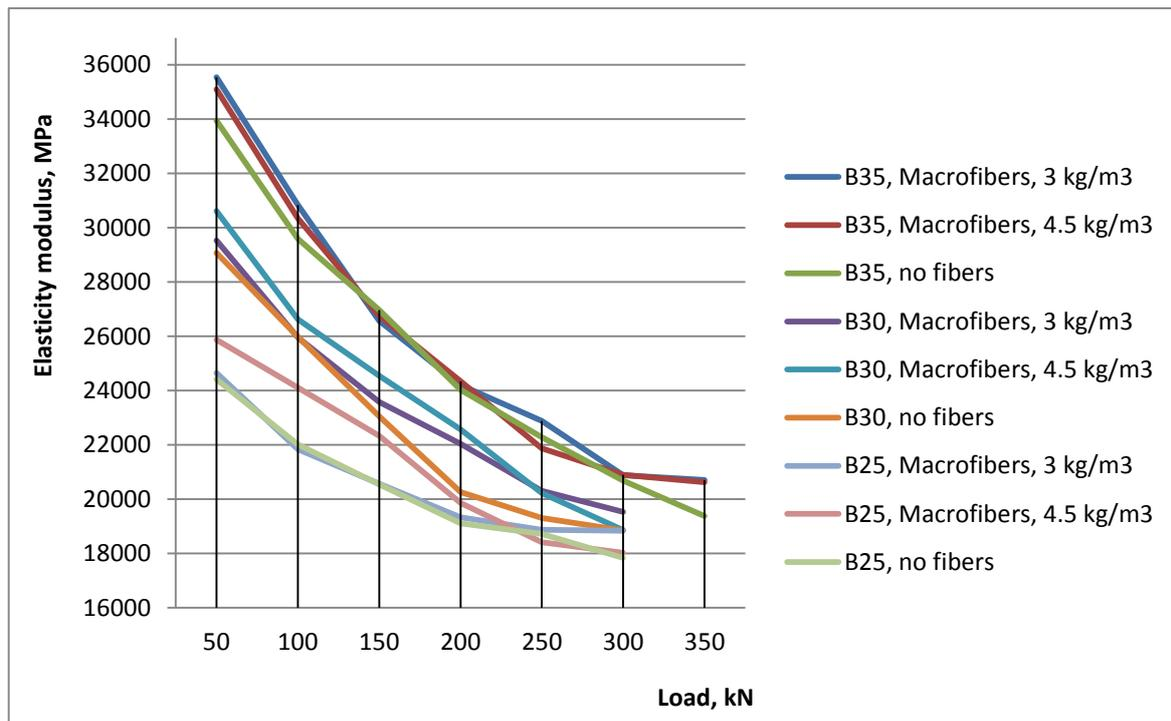
**Figure 8:** Determination of elasticity modulus
