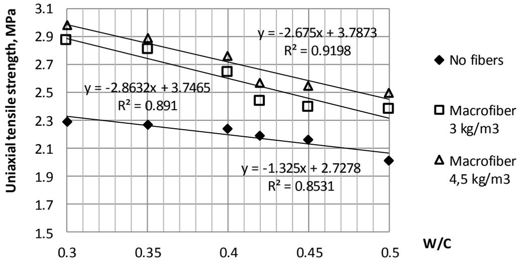
Figure 5: Uniaxial tensile strength at the age of 28 days
