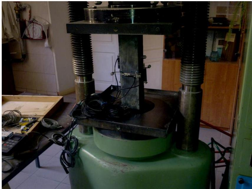
**Figure 7:** Determination of elasticity modulus and Poisson's coefficient
