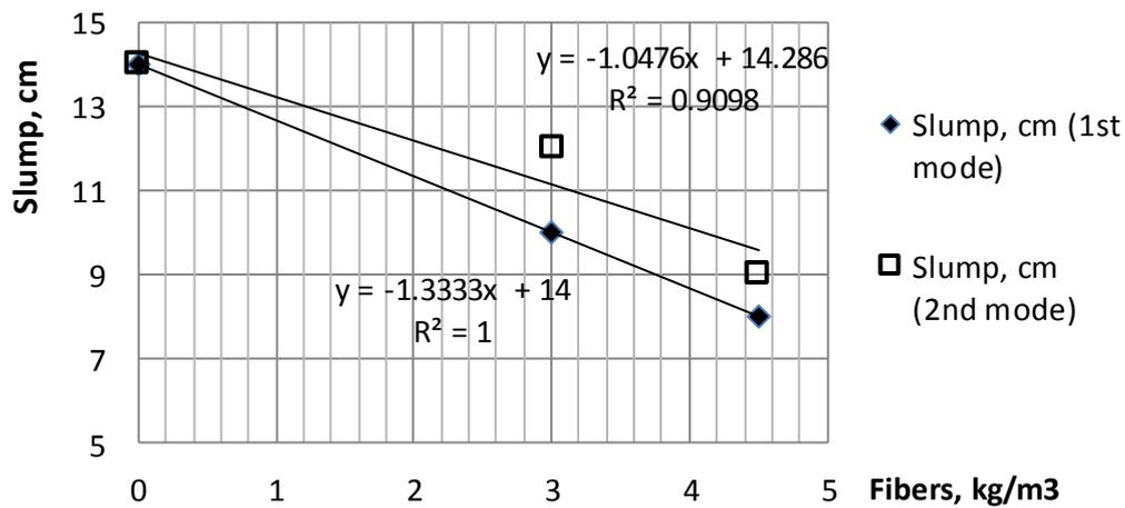
**Figure 2:** The dependence of fresh concrete workability from the macrofibers quantity and mode of macrofibers introduction
