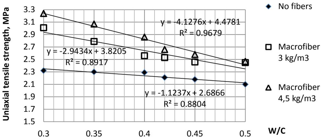
Figure 6: Uniaxial tensile strength at the age of 90 days
