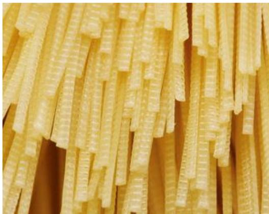
**Figure 1:** The appearance of macrofibers and convenient packing of macrofibers using the water-soluble film
