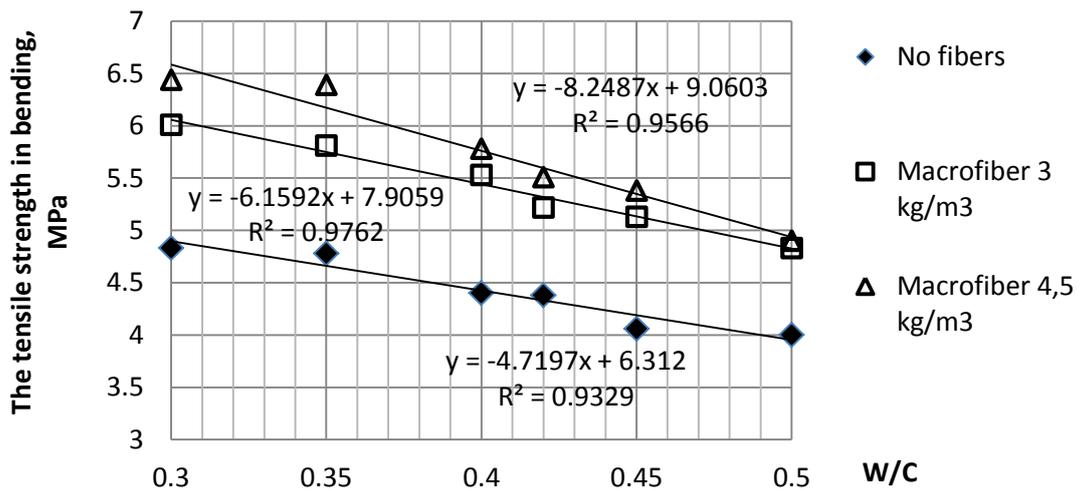
**Figure 4:** The concrete tensile strength in bending at the age of 28 days
