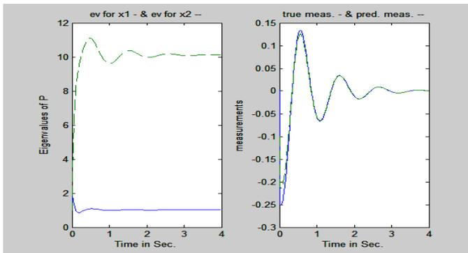
**Figure 2:** Eigenvalues of the P showing convergence/satisfaction of the condition of (10), related to state x1 (-), & state x2 (--); and the true (-), and predicted measurements (--); No missing data.
