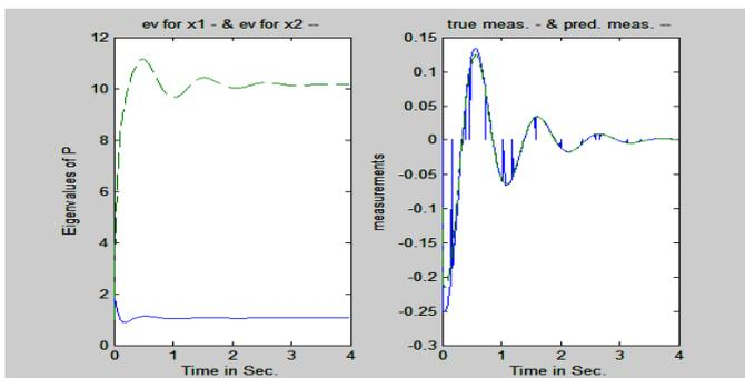
**Figure 4:** Eigenvalues of the P showing convergence/satisfaction of the condition of (10), related to state x1 (-), & state x2 (--); and the true (-), and predicted measurements (--); some missing data.
