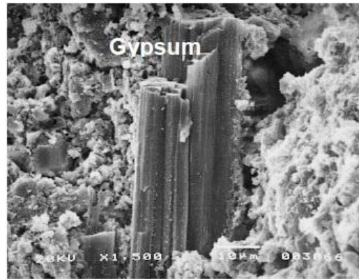
Figure 5b1. SEM micrograph of the BS sample with addition of 3 wt. % VAE after 7 days of hardening
