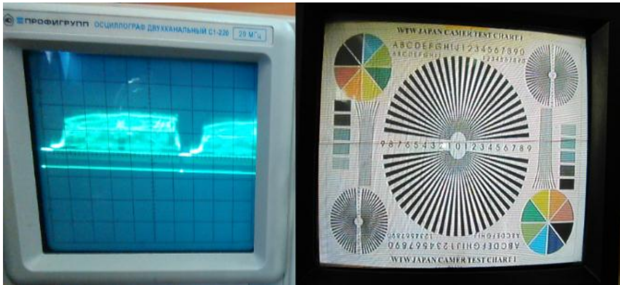
Figure 5: The combined using of a visual (on the right) and the tool (left) control methods for the test table obtained from the monitor by using a TAT-603S, 380 TVL color video camera at illumination with RGB LEDs
