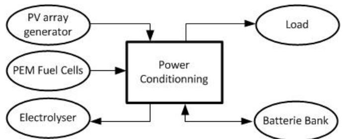
**Figure 1:** Hybrid PV – PEMFC electrolyser system equipped with a battery bank
