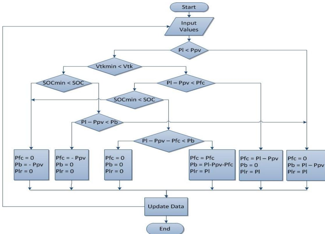
**Figure 3:** Flowsheet diagram of the PV-PEMFC hybrid system energy management
