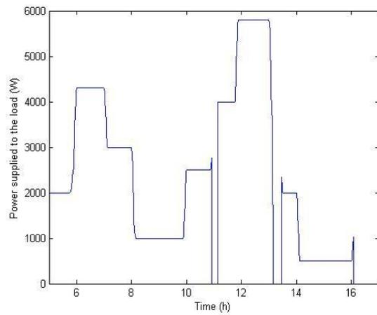
B2) Stand-alone hybrid PV-PEMFC generator power supplied to the load
