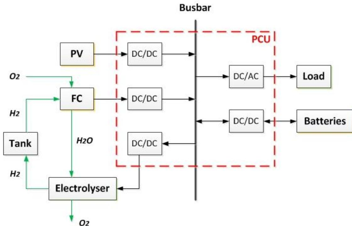
Figure 2: Hybrid PV – PEMFC Topology
