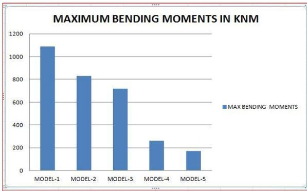
**Figure 9:** Maximum Column bending Moments graph of All Models
