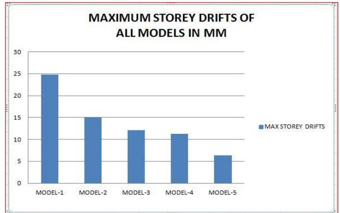
**Figure 8:** Maximum Storey drift graph of All Models
