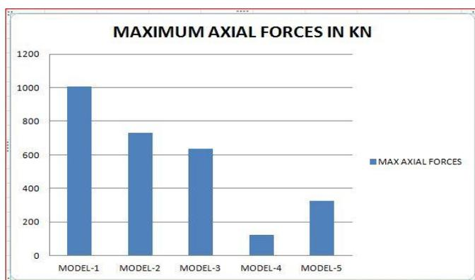
**Figure 10:** Maximum Column Axial forces graph of All Models
