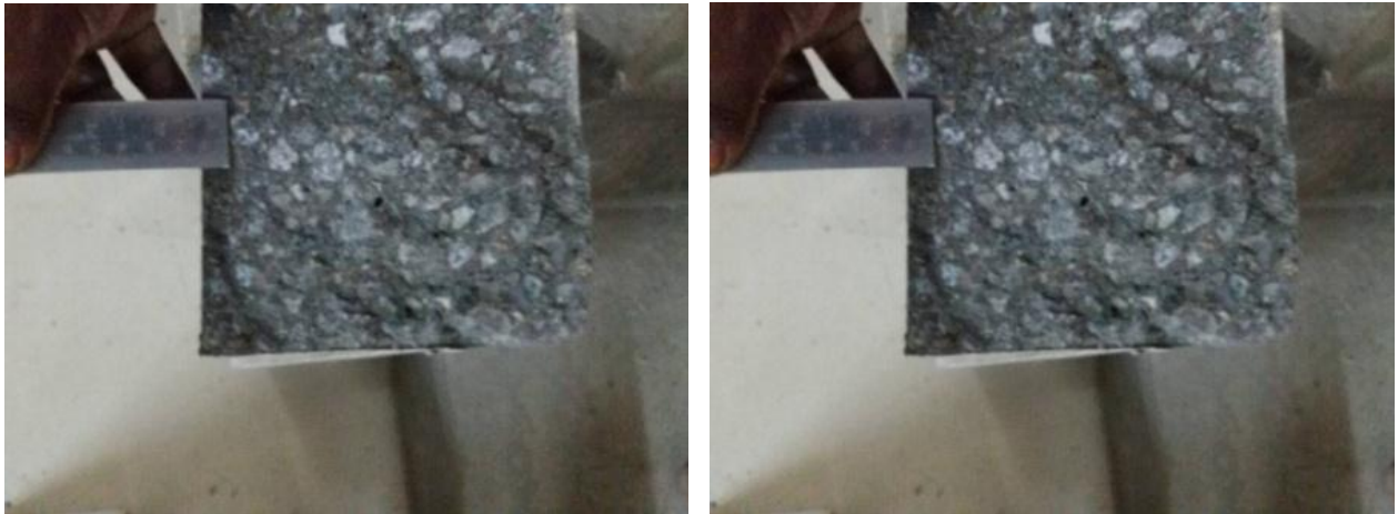
Figure 1: Measuring depth of water penetration
