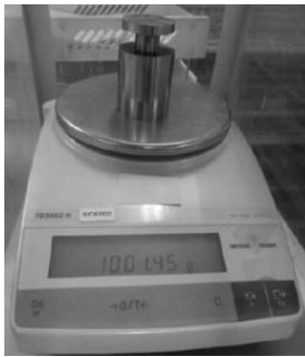
Figure 10: A 1kg experimental standard weight could be read out its measured weight value within the expected safety - range of 1001.453 g – 1001.483g
