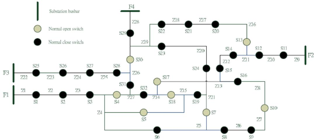
**Figure 5:** The IEEE standard distribution network before reconfiguration under study
