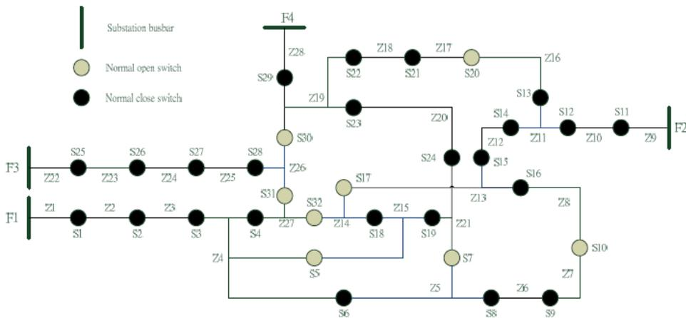
**Figure 6:** The IEEE standard distribution network after reconfiguration under study
