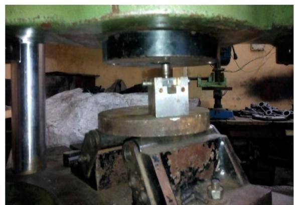
**Figure 6:** The ram and fixture used for ram tensile test.
