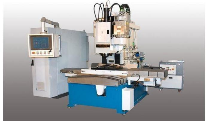
**Figure 3:** Friction surfacing machine used for conducting experiments.
