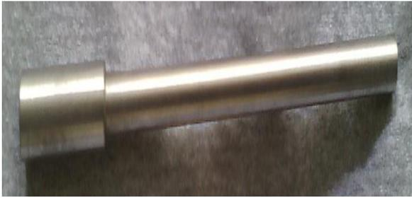
**Figure 2:** Mechtrode before friction surfacing
