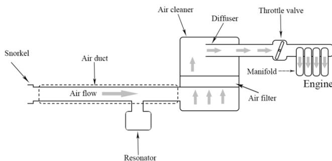
(a) Simple diagram of intake system
