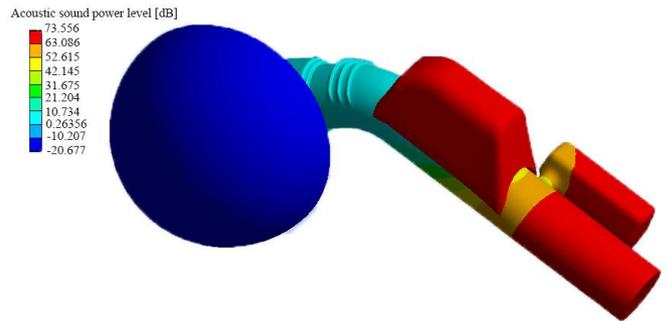
(b) Result of acoustic sound power level at 353Hz
