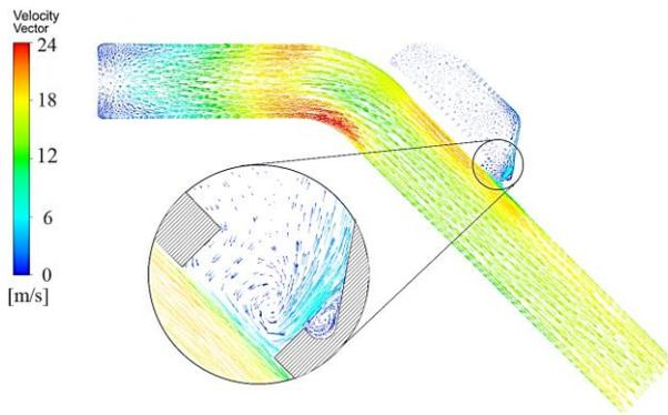
**Figure 6:** Result of velocity vector in cross section of resonator
