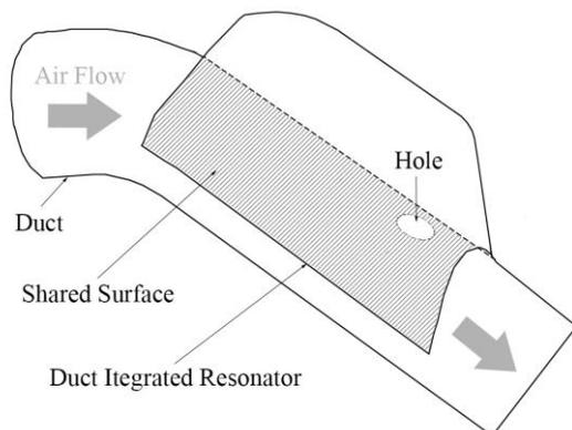
(b) Simple diagram of duct integrated resonator
