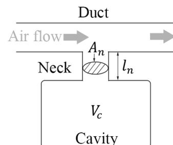
Figure 1 : Simple structural diagram about the Helmholtz resonator
