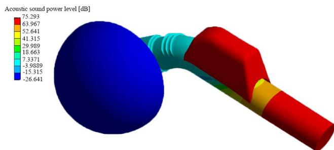
(a) Result of acoustic power level at 350Hz
