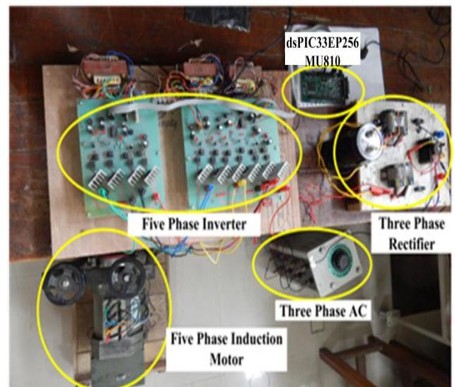
**Figure 5:** Experimental Setup of Five-Phase inverter-motor circuit
