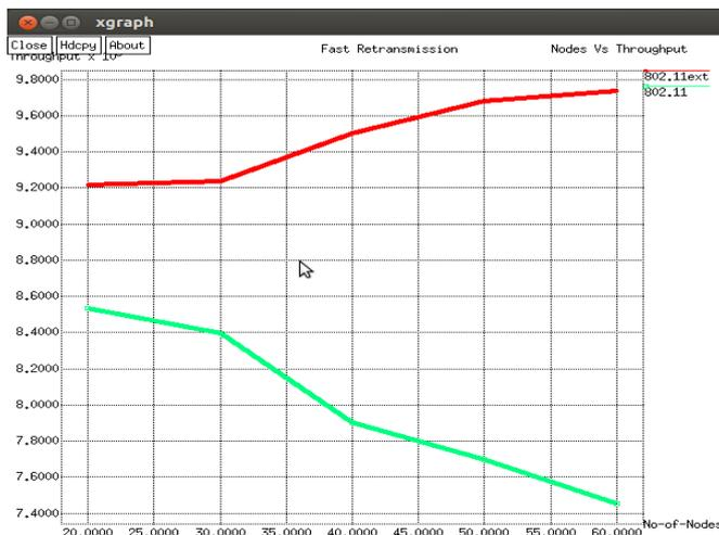
**Figure 5:** Nodes vs Throughput in VANET (IEEE 802.11ext standard) and MANET (IEEE 802.11 standard)
