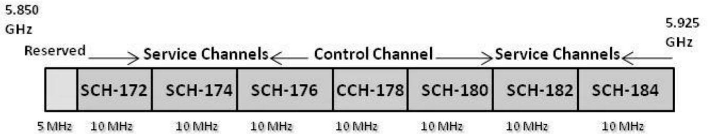
**Figure 1:** Allocation of DSRC Channels
