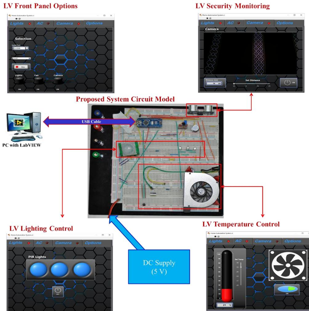
**Figure 3:** Proposed smart home automation system hardware realization.
