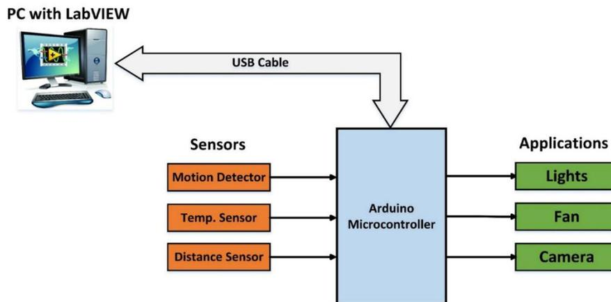
Figure 1: Proposed smart home automation system architecture.
