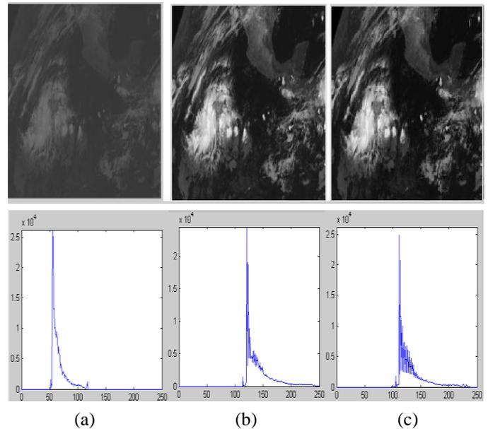
**Figure 2:** Input low contrast image and Output images of different methods with their corresponding histograms.
