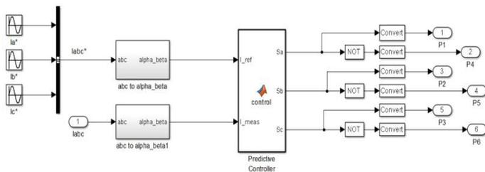
**Figure 4:** Predictive control in DSTATCOM
