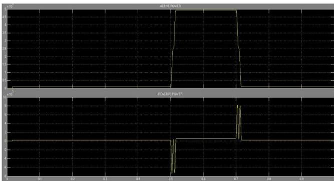
**Figure 6:** Single line to ground fault
