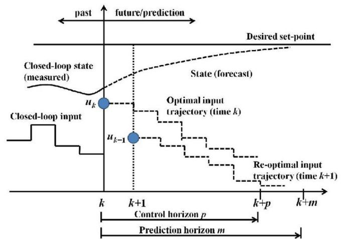
**Figure 2:** Principle of Predictive Control
