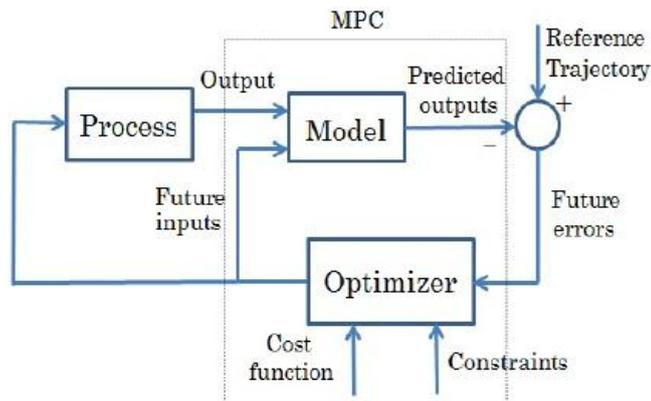
Figure 3: Block diagram of MPC algorithm
