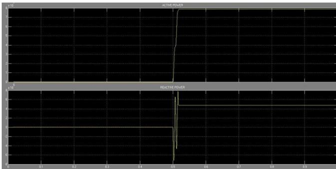
**Figure 7:** Double line to ground fault
