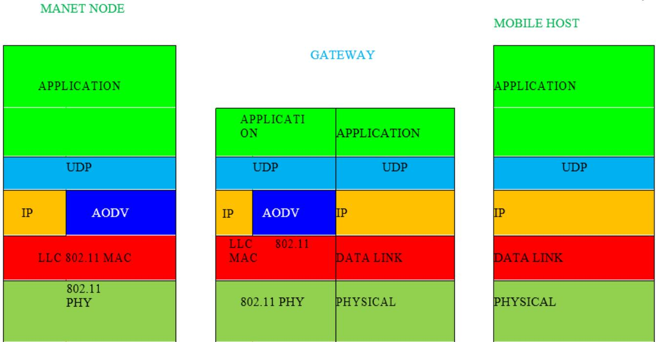
Figure 3: Gateway Protocol Stack: MANET-INTERNET Integration
