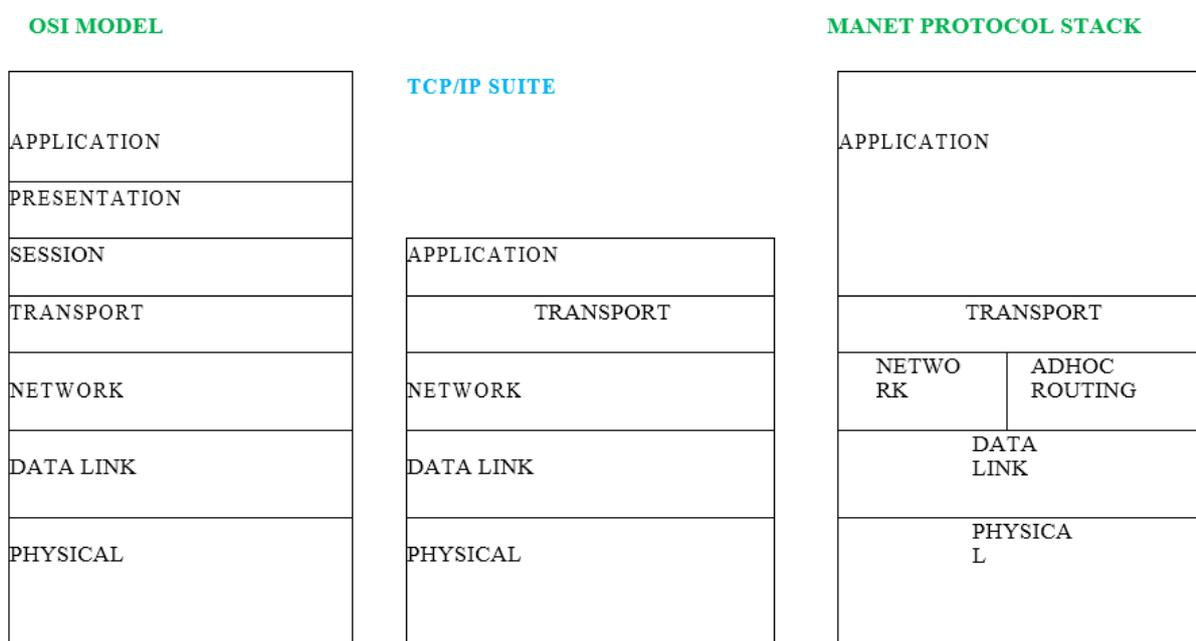
**Figure 2:** Basic Protocol Stack of Network Routing
