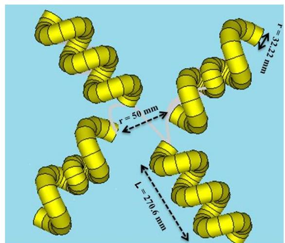
**Figure 9:** Helix Cross dipole antenna
