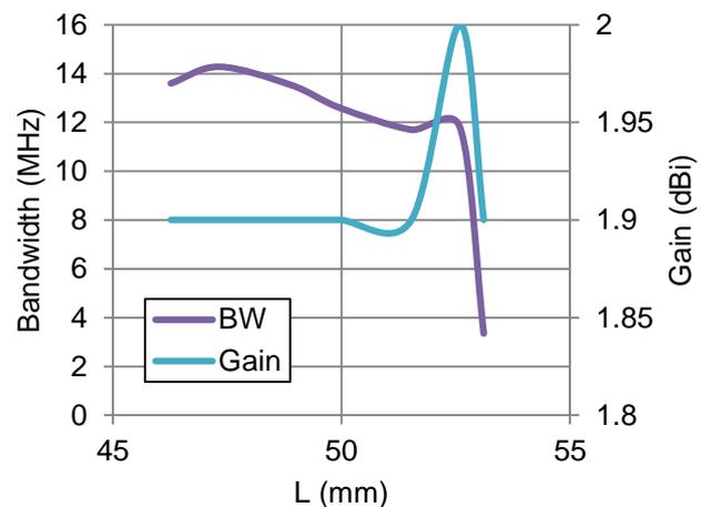
Figure 13: Simulation of bandwidth and gain meander antenna
