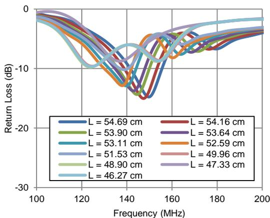
Figure 11: Optimization Meander Antenna Design
