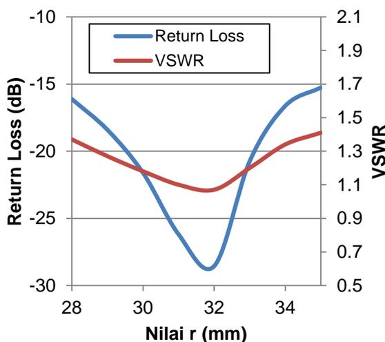
**Figure 7:** The  $r$  value iteration as well as its effect on return loss and VSWR.
