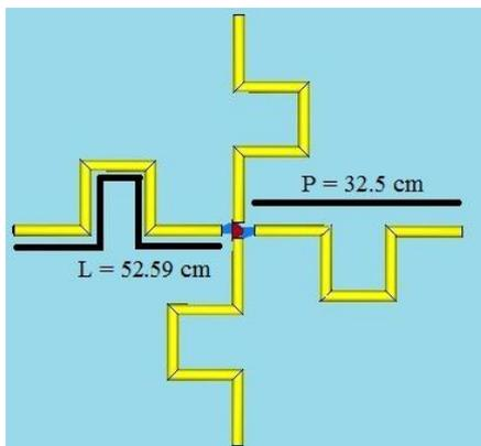
Figure 10: Meander Cross dipole antenna
