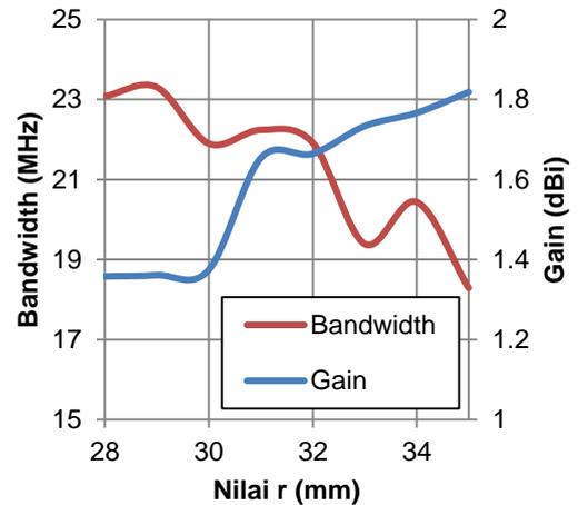
**Figure 8:** Simulation of bandwidth and gain helix antenna
