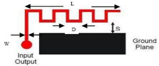
Figure 2: Meander Antenna
