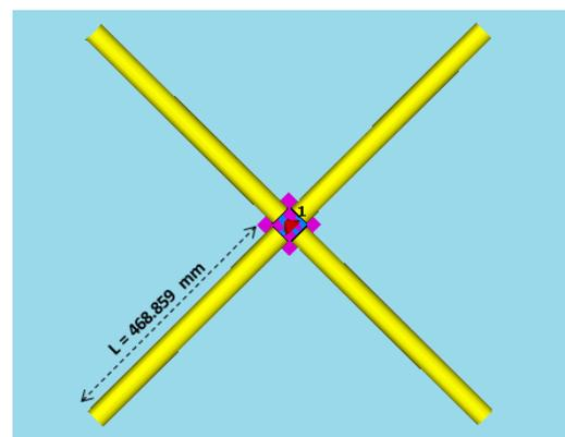
Figure 4: Dimensions of 137.9 MHz cross dipole antenna
