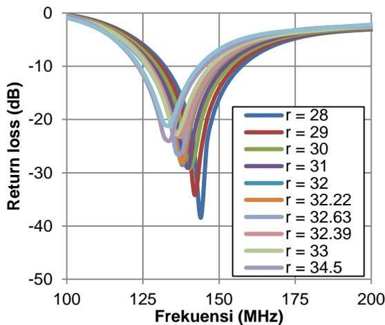
**Figure 6:** Optimization Helix Antenna Design
