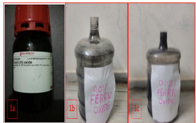
Figure 1a: Ferric Oxide Nano Powder, Fig.1b Nano fluids 0.01% concentration, Fig.1c. Nano fluid 0.03% concentration
