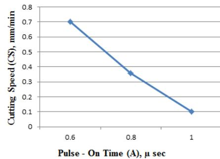
From the above fig the maximum value of Pulse-on time i.e.  $A = 1.0 \text{ sec}$ , is taken as the pulse-on time value for further experiments conducted to improve the cutting speed (CS).
