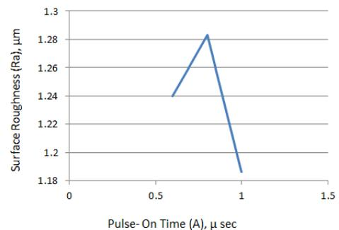
**Pulse-On time (A) Vs. Surface Roughness**
