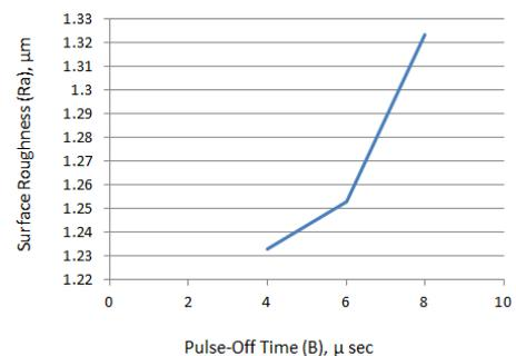
**Pulse-Off time (B) Vs. Surface Roughness**
