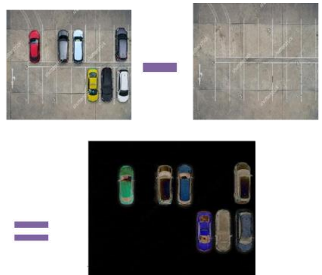
Figure 9: Subtraction of initial park status from current image status
