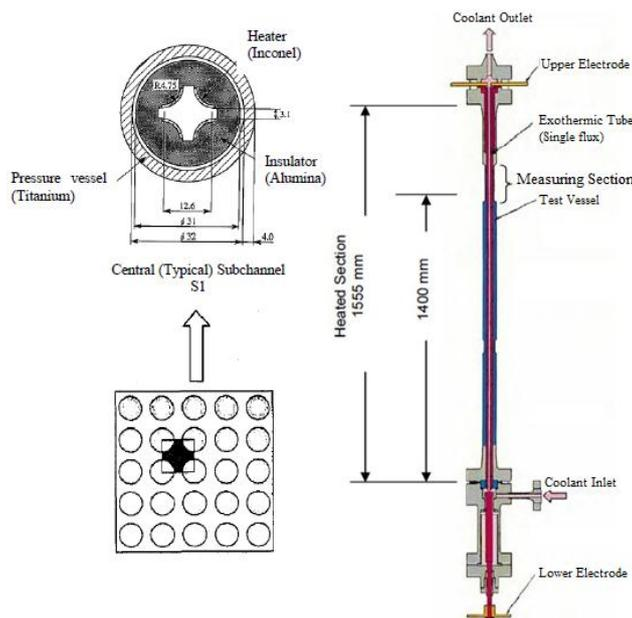
**Figure 3:** Cross-sectional View of Central (Typical) Subchannel Test Assembly [3]
