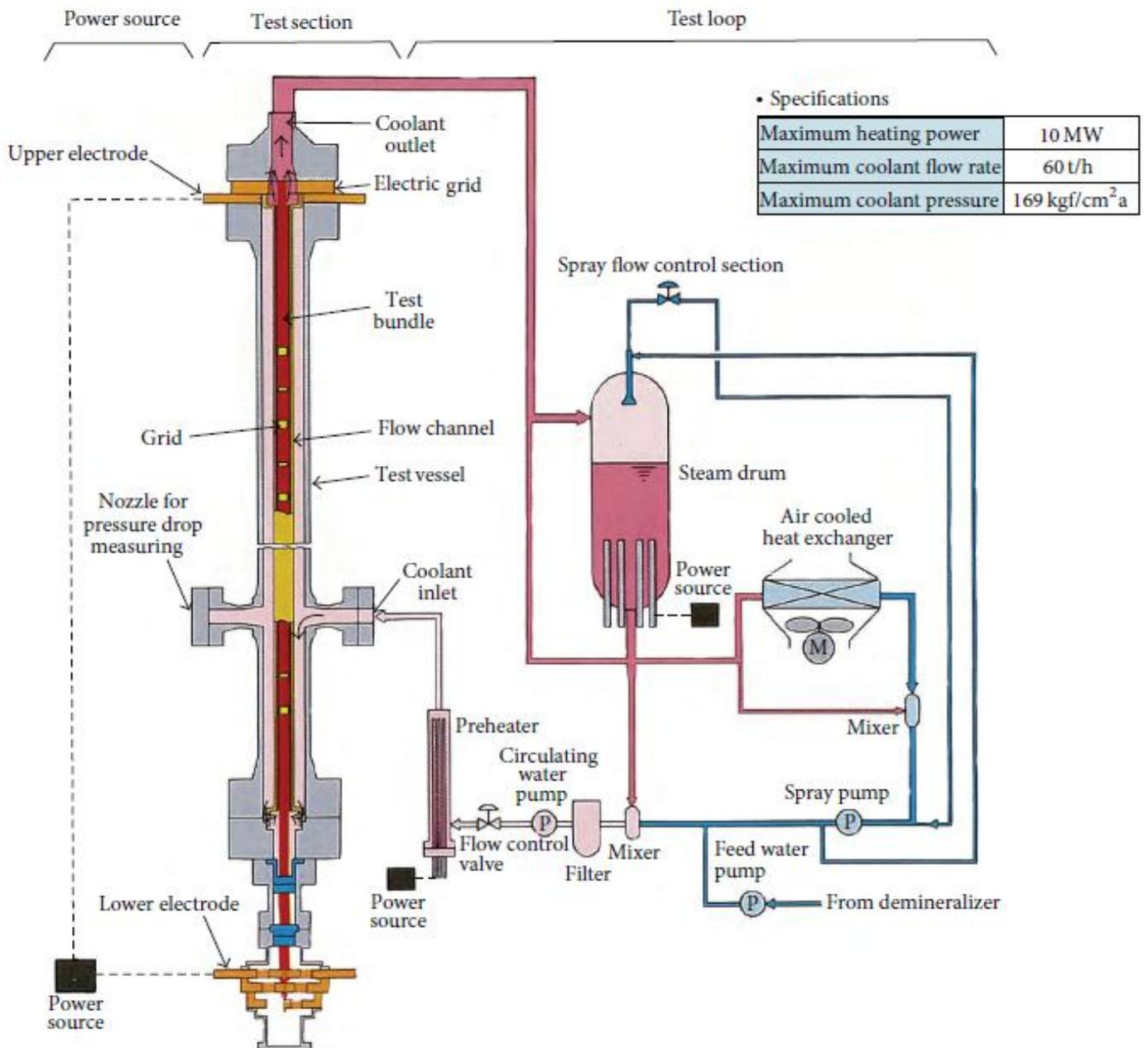
Figure 1: System Diagram of NUPEC PWR Test Facility [3]
