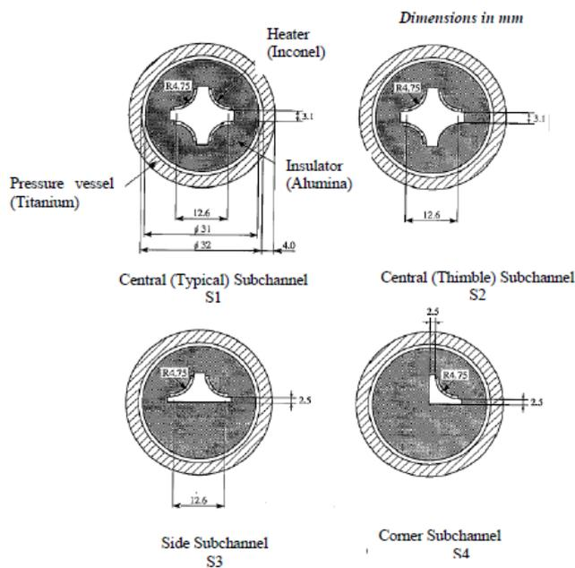
**Figure 2:** Cross-sectional View of Subchannel Test Assembly [3]
