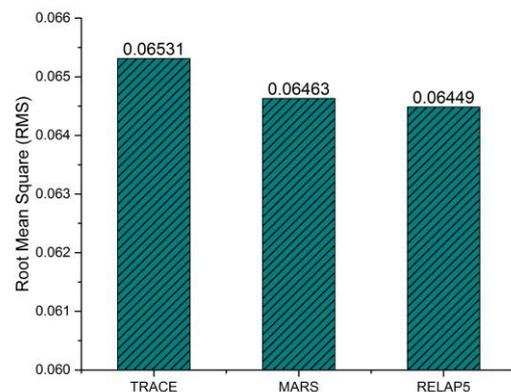
Figure 7: Root mean square values for TRACE, MARS-KS, and RELAP5
