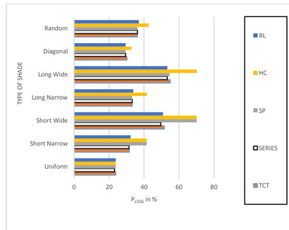
Figure 6(b): shows the plots between P<sub>Loss</sub>% under different shading patterns for different interconnections
