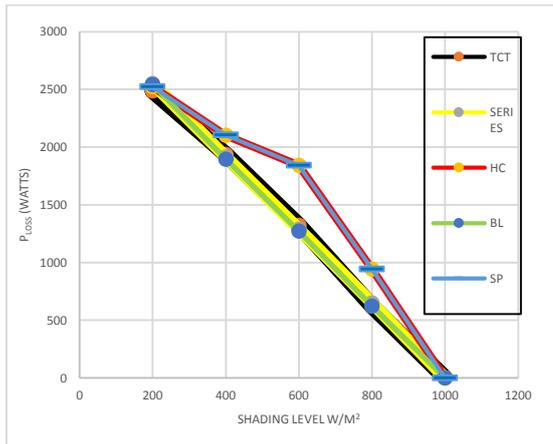
Fig. 5. shows the plots between losses against shaded panel insolation under different shading levels for different interconnections
