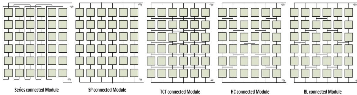
**Figure 2:** Module Connection Topologies.
