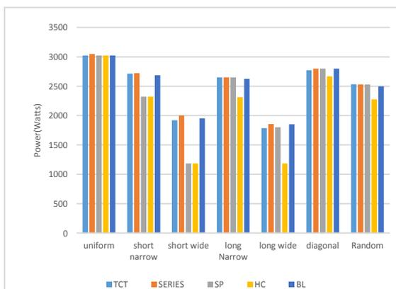
Figure 6(a): shows the plots between Power outputs under different shading patterns for different interconnections.
