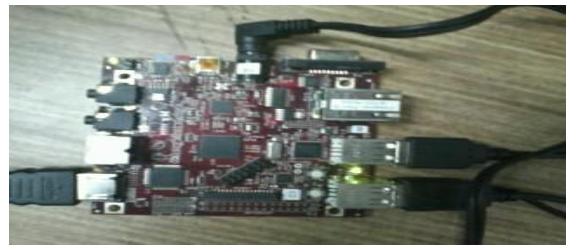
Figure: Hardware Kit of Beagle board-xM
