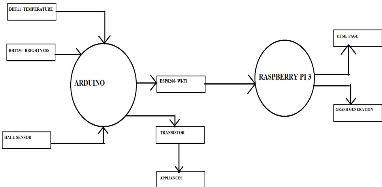
**Figure 2:** Data Flow Diagram
