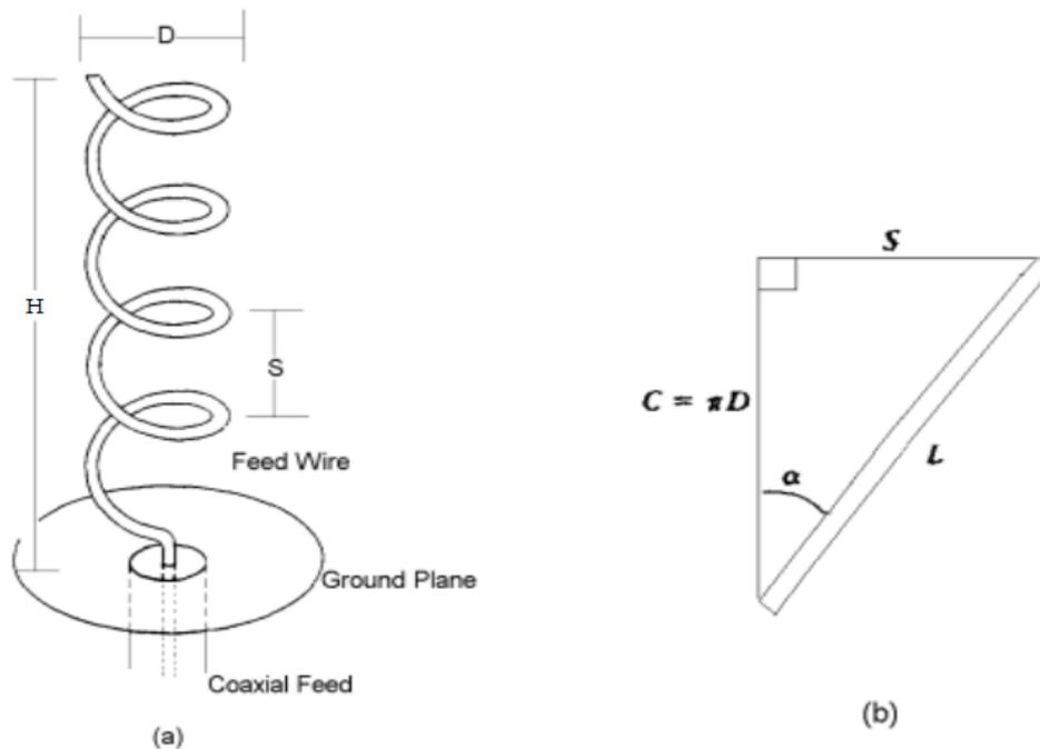
**Figure 1.** a) Geometry of antenna; b) Unrolled turn of antenna [5]
