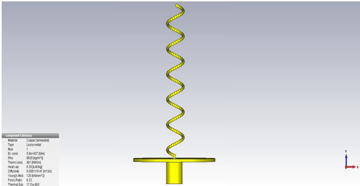
**Figure 2.** Helical antenna
