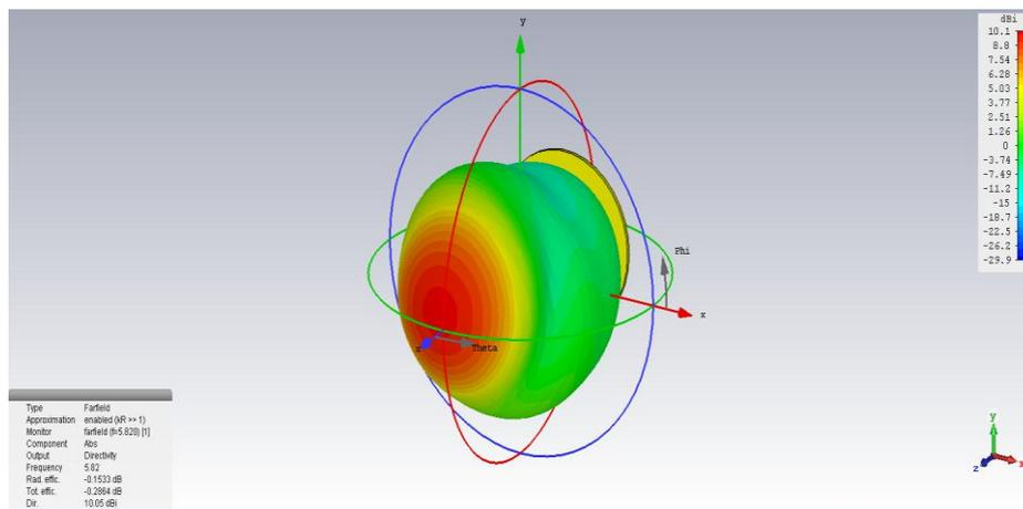
**Figure 7.** Radiation of Helical Antenna in Far-Field – Directivity
