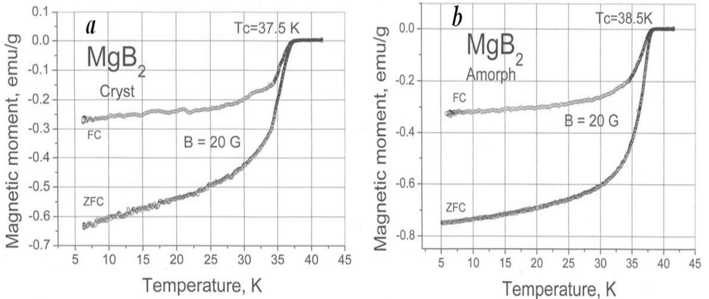
**Figure 4:** Temperature dependences of the zero-field cooled (ZFC) and field-cooled (FC) magnetic moment for HEC  $MgB_2$  composites at 1000 °C with intensity of loading 10 GPa in magnetic field 20 Oe
