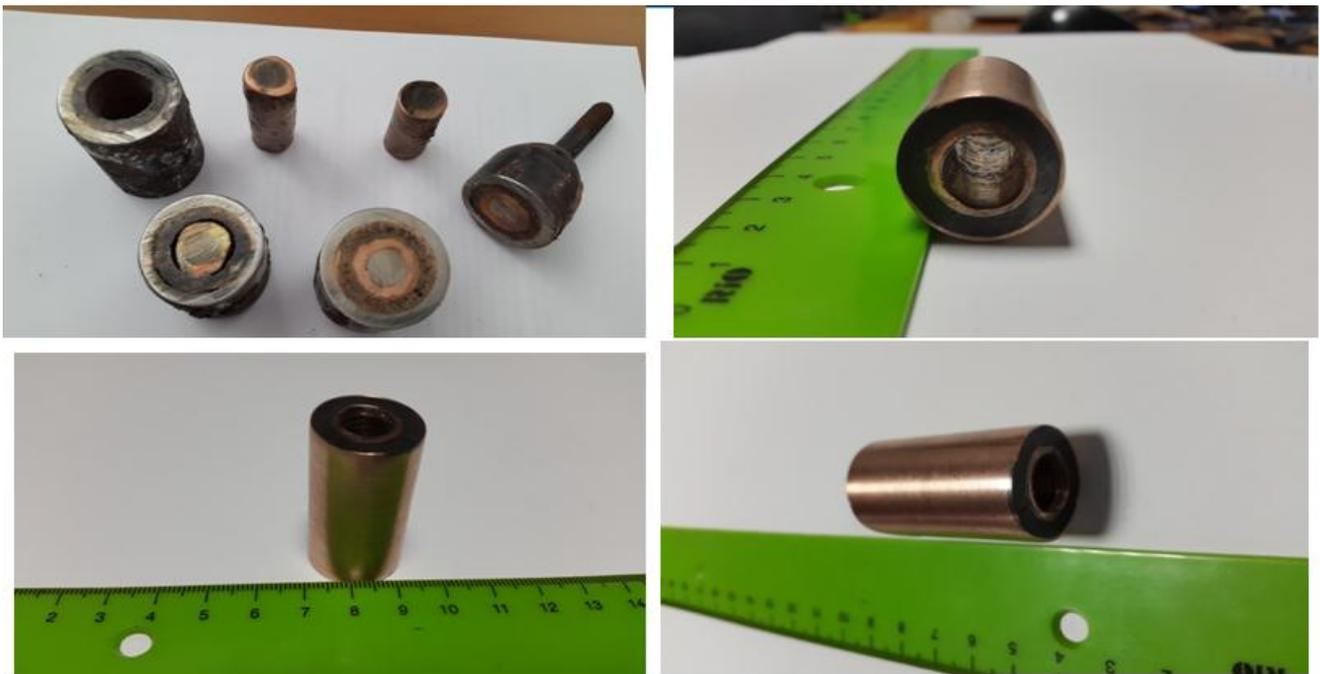
**Figure 7:** Cu-MgB<sub>2</sub>-Cu superconductive tubes
