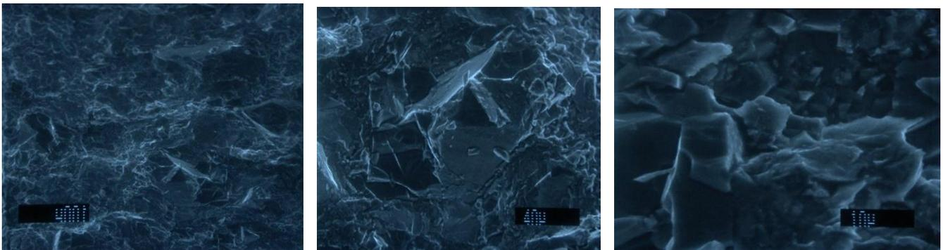
**Figure 5:** Microstructures of the HEC  $MgB_2$  composites HEC at 1000°C and loading intensity 10 GPa from pure Mg and B powder blends [6]
