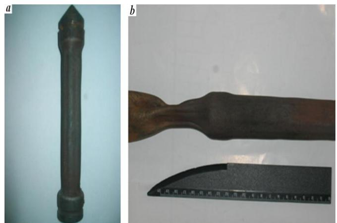
**Figure 3:** Views of billets before (a) and after the HEC procedure at 1000 °C and loading intensity 10 GPa (b)
