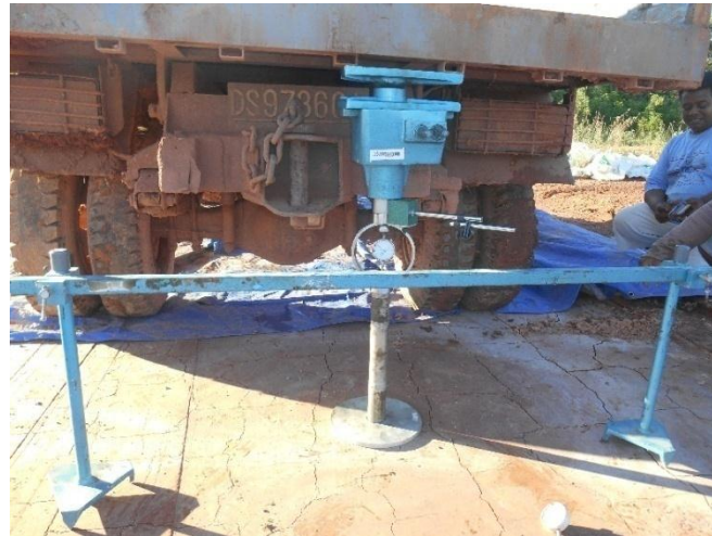
Figure 3. Field CBR testing equipments
