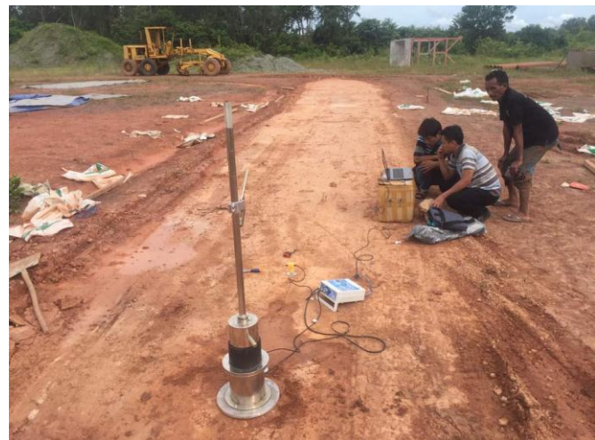
Figure 4. LWD test for measuring the deflection at the field
