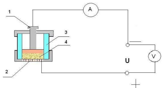
**Figure 1:** 1 – anode, 2 – cathode, 3 – the case from insulating material, 4 – research environment, A – ampermeter, V – voltmeter
