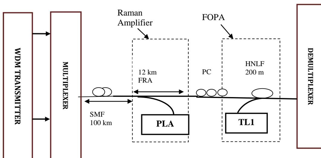
**Figure 1:** Schematic for Experimental set up. FRA-Fiber Raman Amplifier, PC- Polarization Controller, PLA-Pump laser Array, TL-tunable laser
