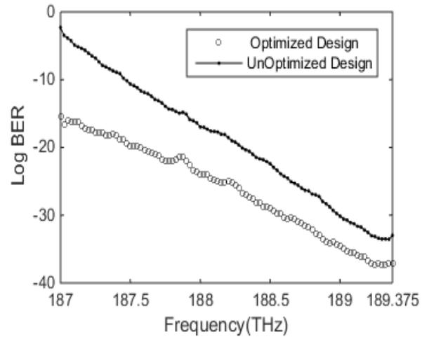
**Figure 5b:** Log BER comparison for Optimized and Un-optimized pump powers
