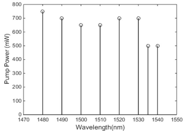
**Figure 2a:** Raman pump powers for un-optimized 96 channel DWDM system
