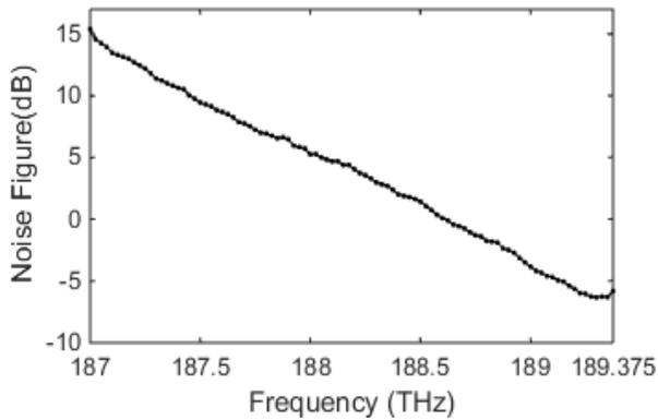
**Figure 3b:** Noise Fig. variations of the proposed hybrid using un-optimized pump powers
