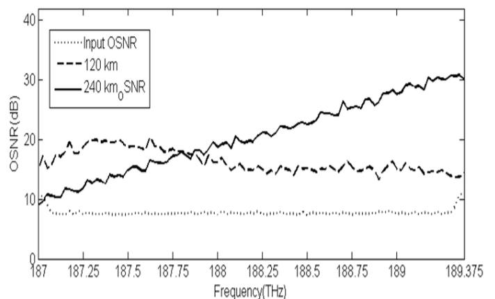
**Figure 3a:** OSNR variations for 2-stages amplification using un-optimized pump powers
