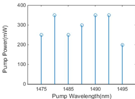
**Figure 4:** Optimized Raman pump wavelengths and their powers for proposed system
