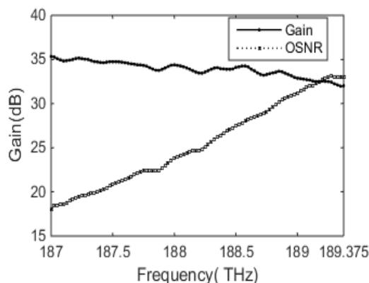
**Figure 5a:** Gain and OSNR Variations for optimized Raman pump powers over transmission distance of 300 km
