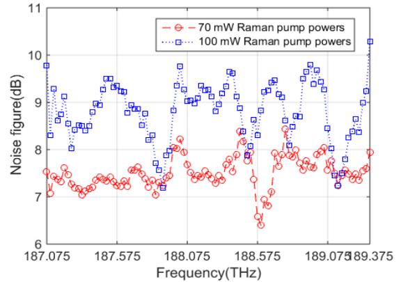
**Figure 3b:** Noise Fig. variations for Raman-FOPA hybrid with Raman fiber length 10 km and FOPA length 0.5 km. at different Raman pump powers.
