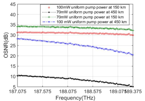
**Figure 4a:** OSNR comparison for Raman-FOPA with varying pump power of Raman amplifier at 70mW and 100 mW over distance of 450 km at  $P_{in}$  of 3mW
