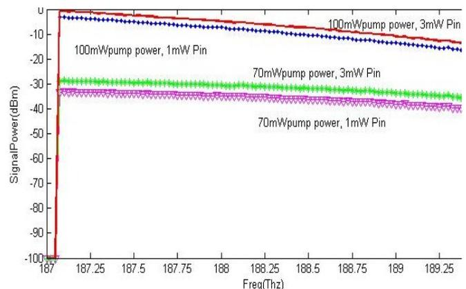
**Figure 4b:** Signal Power comparison for Raman-FOPA with Varying pump power of Raman amplifier at 70mW and 100mW over distance of 450km with each fiber span of 75km at  $P_{in}$  of 3mW and 1mW.
