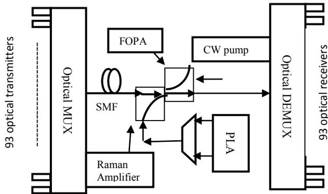
**Figure 2.** DWDM Schematic for setup of FOPA and Raman-FOPA analysis
