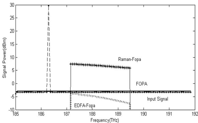
**Figure 1.** Signal power of FOPA, FOPA-EDFA and RAMAN –FOPA compared with input to the fiber
