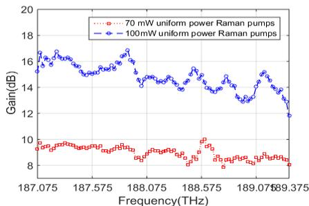
**Figure 3a:** Gain variations for Raman-FOPA hybrid with Raman fiber length 10 km and FOPA length 0.5 km. at different Raman pump powers.
