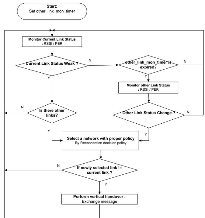
Figure 2: Vertical handover procedure
