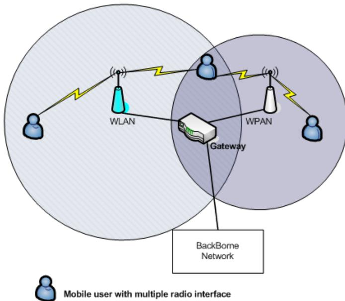
Figure 1: An overlaid network using both WLAN and WPAN
