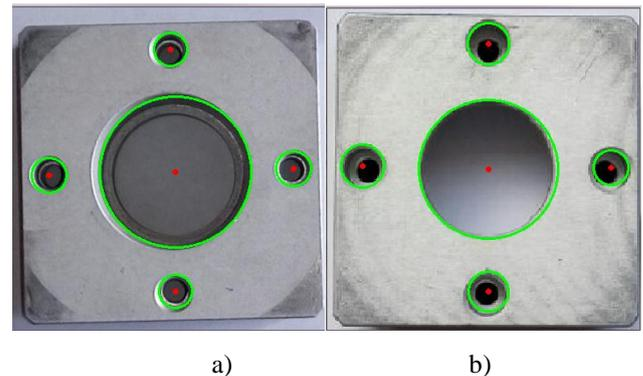
**Figure 6:** a) Straight Piece Detection. b) Backwards Piece Detection.
