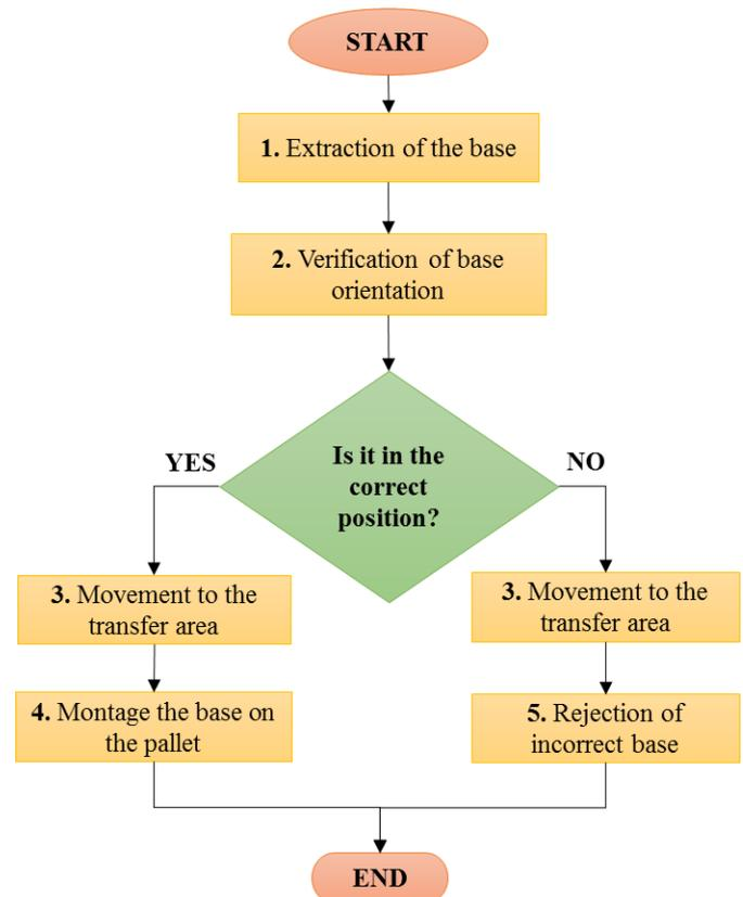
**Figure 3: Process Flow Diagram**
